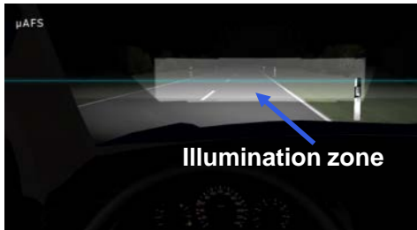
μAFS (solid state-lighting) ~4.000 Pixel
