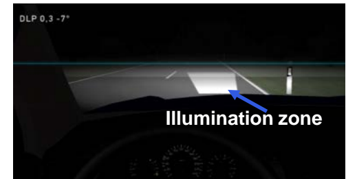
DLP (Digital Light Projection) >500.000 Pixel
